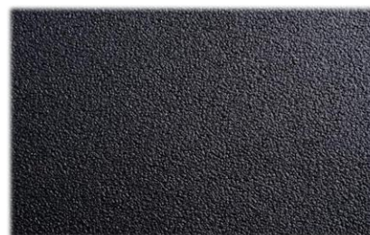
Texture effect in solvent-based systems can be achieved using the MEGH™PRINT W grades; 3% dosage
