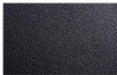
Texture effect achieve with MEGH™PRINT P 45 texture additive; 3% dosage
