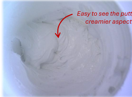
PVA internal wall putty, with 0,7% of MEGH™WAX EEW 5030, an Ester wax emulsion 45%,
