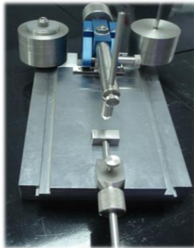
machine used to measure scratch "sclerometer"
