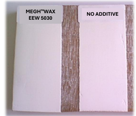
Application of MEGH™WAX EEW 5030, an Ester wax emulsion 45%, in a PVA internal wall putty
