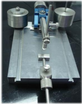
machine used to measure scratch “sclerometer”
