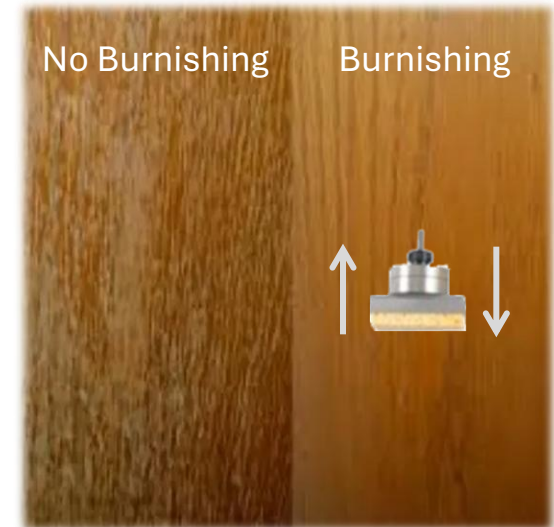
Typical wood coating subjected to burnishing
